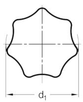
$\begin{array}{lll} d1 & = 50 \\ d2 & = M \ 10 \\ d3 & = 18 \\ h1 & = 32 \\ h2 & = 15 \\ t1 \ min & = - \\ Weight in (g) = 210 \\ \end{array}$
